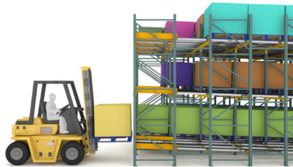
Square the forklift with lane & raise the pallet 3" above the rails
