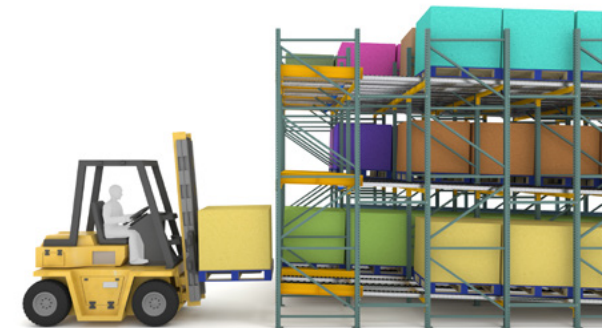
Follow the same process to load the remaining pallet positions
