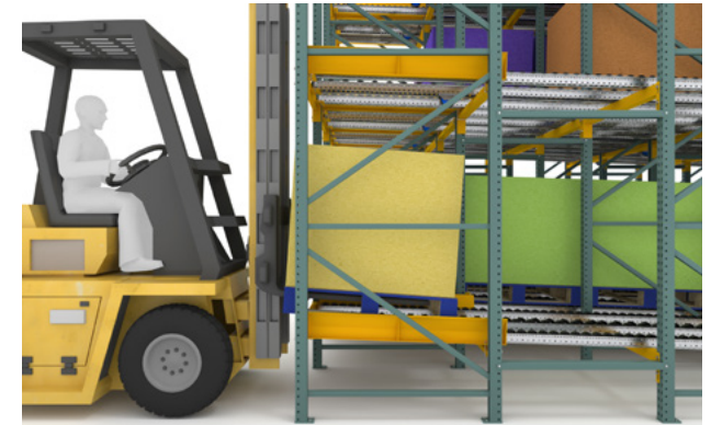
Place the pallet centered in the lane & tilt onto the rails
