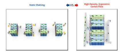
Carton flow functions with separate load and pick aisles, allowing the two functions to occur concurrently. Cases, totes, or single items flow from the charge side down to the pick aisle on slightly inclined rails.
